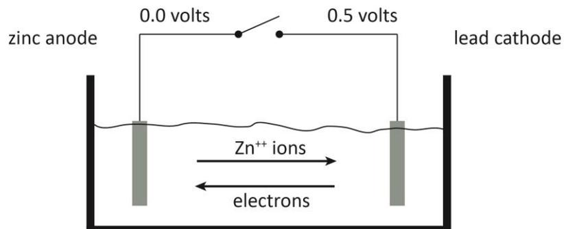
The diagram above shows an example of a reaction between a zinc anode and a lead downrigger ball when both are immersed in seawater. If the zinc and the downrigger ball are not electrically connected within the boat the anode will release zinc ions (positively charged zinc atoms) while the downrigger ball will release electrons, until a charge builds up on both. Once the charge has built up the result is an
